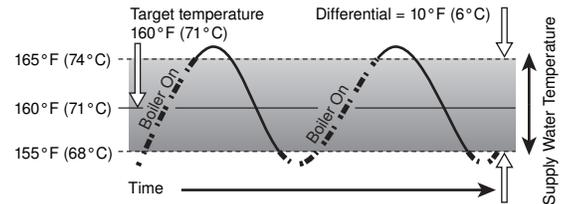
When the boiler is modulating above low fire, the differential does not apply. Instead, the modulation output signal is determined using Proportional, Integral and Derivative (PID) logic in order to satisfy the boiler target temperature.
