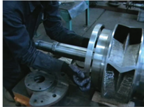
Picture 4 – Neck Ring Installation
