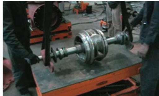
Picture 2 – Rotating Assembly
