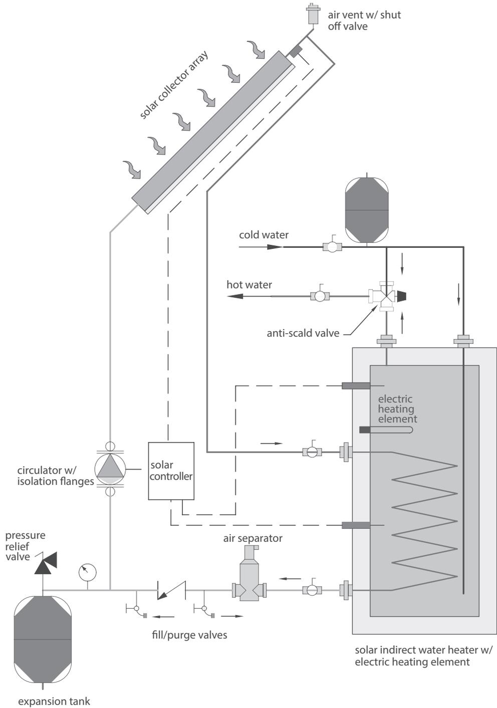
Figure 3: Single tank system with electric backup
