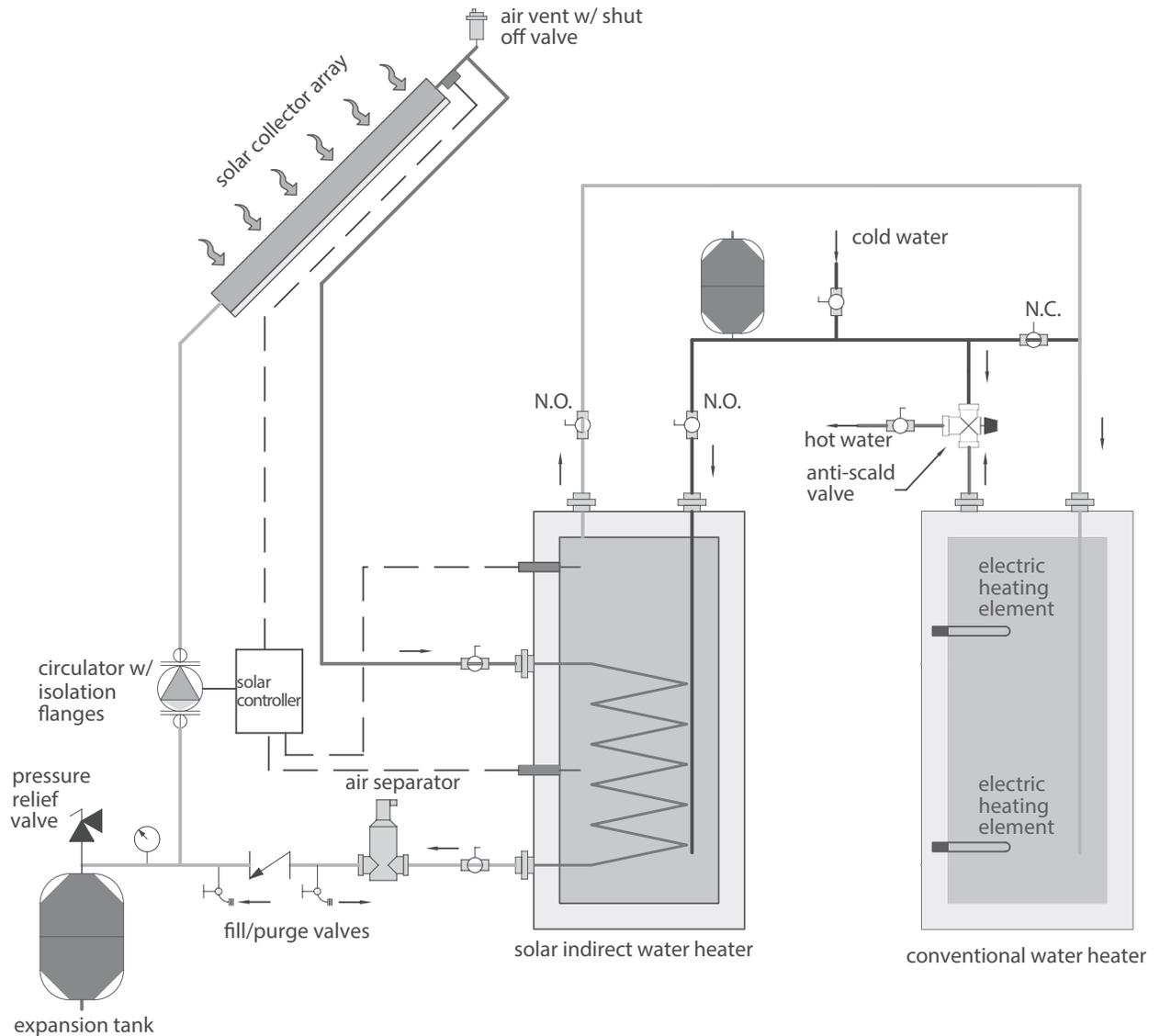
Figure 4: Two tank system with existing heater
