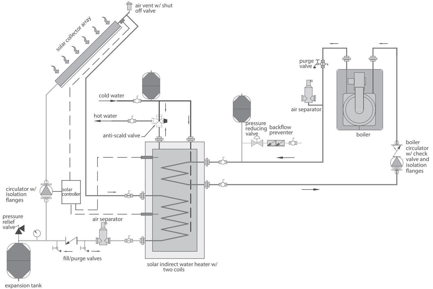
**Figure 5:** Single tank system with boiler backup
