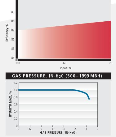
The Futera III provides high tolerance for real world conditions as it maintains 100% full input down to 2"wc.
