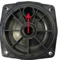
The arrow indicates the top side of the HU25. The HU25 should only be used in this orientation with the pressure outlet at 12 o'clock.
