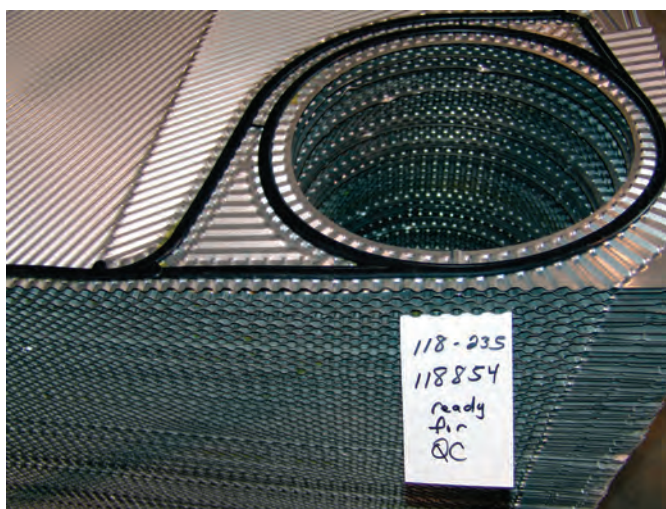
Plates are pressed in virtually any cold-formable metal and furnished with the right gasket materials to match your process conditions.
