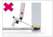
It is the responsibility of the installing contractor to verify compatibility of any chemicals that come into contact with the PPSU fittings. In addition, the installing contractor should ensure that other trades on the job site do not allow external chemicals to come into contact with the PPSU fittings. If it is required to protect the fittings, use only REHAU recommended protective tapes for wrapping of EVERLOC+ joints.
