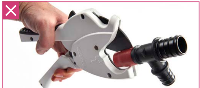
Fig. 4.10: DO NOT cut RAUPEX pipe from fitting
