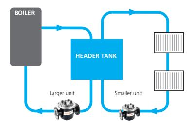
BoilerMagXT is typically installed on the return circuit as close to the boiler as possible. On larger systems, such as the one shown, smaller BoilerMagXT units may be installed elsewhere to give extra protection for radiators and pipework.
