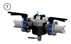
If required open the vent shown on the top of the unit to release any trapped air\*.
