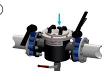
When the draining water runs clear turn off the inlet isolation valve and allow the remaining contents to drain. Close the drain valve and replace the plug.
