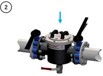
Remove the black tricone positioned on the lid.
