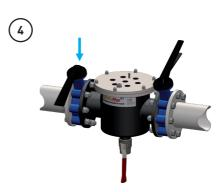
Either place a bucket underneath or connect a hose to the 1¼" drain valve on the underside of the BoilerMagXT. Remove the drain plug and open the drain valve. Partially open the inlet isolation valve and allow the contents to drain through the drain valve.
