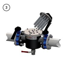
Lift out the magnetic cores using the handle on top of the unit. \*Warning see below\*. Be careful not to place the cores on or near ferrous items.
