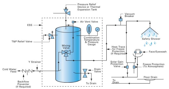
NOTE: For systems requiring recirculation see ThermOmegaTech® IMI for typical piping schematic.
